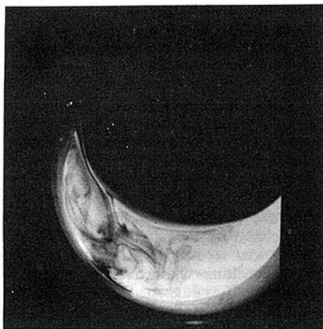
Fig. 5 Visualized flow structure for ice, T_w = 12^\circ\text{C} , t = 16 \text{ min } 15 \text{ s}
